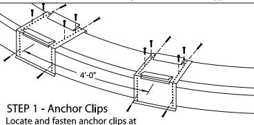
4'-0" O.C. with provided fasteners for substrate using the third full hole from bend (see detail A).
