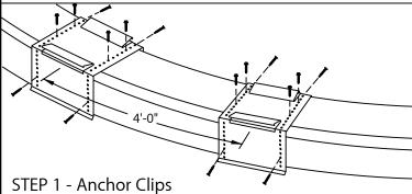
Locate and fasten anchor clips at 4'-0" O.C. with provided fasteners for substrate (see detail A).
