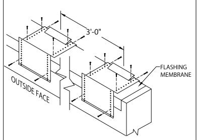
STEP 7 - ANCHOR CLIPS LOCATE AND FASTEN GALVANIZED ANCHOR CLIPS TO WALL AT 3'-0" CENTERS WITH PROVIDED FASTENERS FOR SUBSTRATE (SEE DETAIL A).
