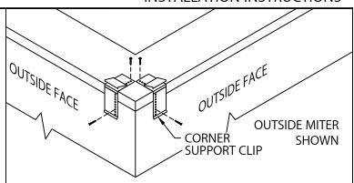
STEP 1 - CORNER SUPPORT CLIPS LOCATE AND FASTEN GALVANIZED CORNER SUPPORT CLIPS TO THE WALL.
