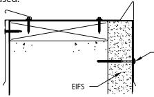
If using an EIFS system, fasten through face w/ fastener of proper length to penetrate through EIFS and attach into structural component
