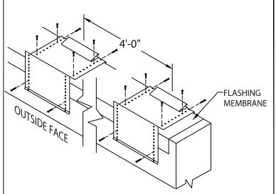
STEP 7 - ANCHOR CLIPS LOCATE AND FASTEN GALVANIZED ANCHOR CLIPS TO WALL AT 4'-0" CENTERS WITH PROVIDED FASTENERS FOR SUBSTRATE (SEE DETAIL A).
