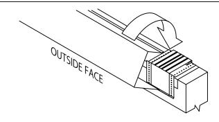
STEP 9 - COPING HOOK OUTSIDE FACE OF COPING OVER THE ANCHOR CLIPS AND ROTATE INTO PLACE. ENGAGE REAR LEG ONTO ANCHOR CLIPS BY PRESSING DOWNWARD UNTIL SNAP LOCK OCCURS.
