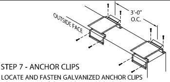
LOCATE AND FASTEN GALVANIZED ANCHOR CLIPS TO WALL AT 3'-0" CENTERS WITH PROVIDED FASTENERS FOR SUBSTRATE (SEE DETAIL A).
