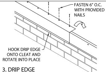
HOOK DRIP EDGE OF EACH DRIP EDGE SECTION ONTO CONTINUOUS CLEAT, ROTATE INTO PLACE. FASTEN THRU PRE-SLOTTED HOLES 6" WITH PROVIDED NAILS.
